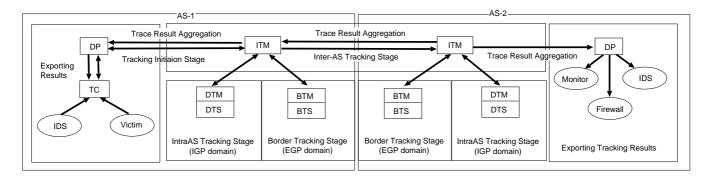
Figure 3: Procedures of an attack tracking on InterTrack
